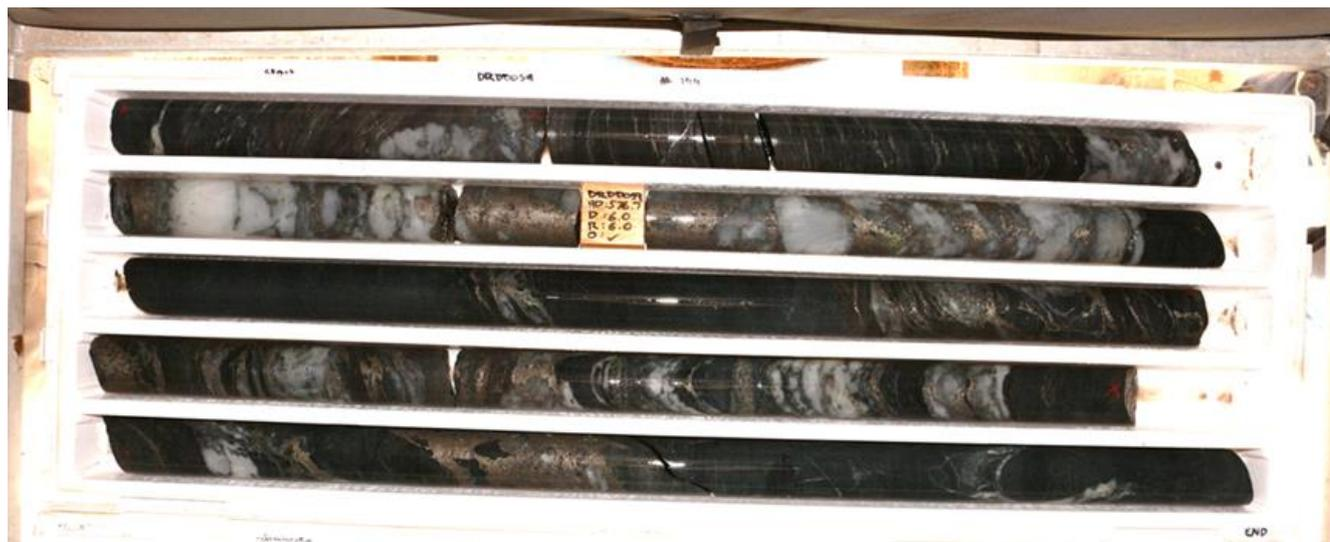
**Figure 1:** DRDD059 diamond drill core mineralised intersection with semi-massive pyrrhotite and brecciated quartz similar in style and widths to the Bellevue Lode. Abundant fine grained visible gold is observed in the mineralised interval.
