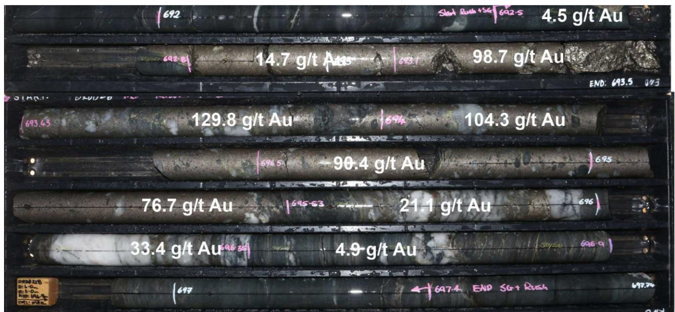
Figure 2: Deacon high grade ore shoot-massive pyrrhotite with trace chalcopyrite, quartz clasts and numerous visible gold grains in DRDD218. Interval assayed 4.4m @ 62.4 g/t gold from 692m.
