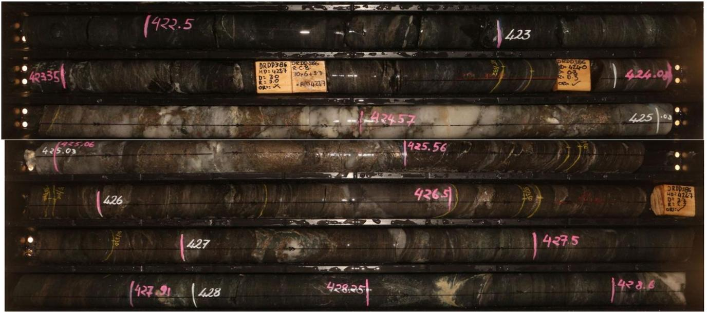
**Figure 3: DRDD396 Large quartz vein of intermixed smokey and milky quartz with minor chlorite/biotite shearing on margins. Pyrrhotite 5% and trace chalcopyrite occurring as fracture fill/cataclastic with minor stringer veins. 17+ specks of visible gold dispersed throughout the interval. Assays pending**
