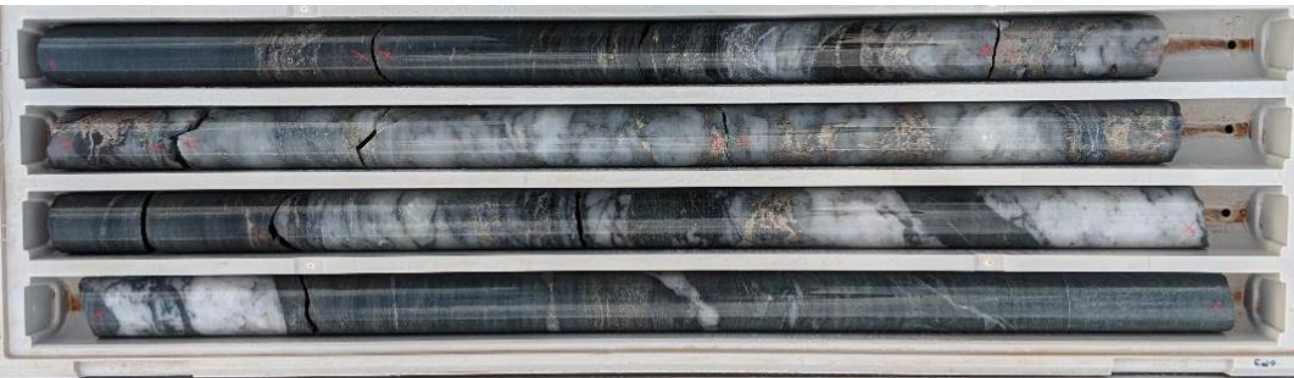
Figure 3: Recent drill hole DRDD089 Bellevue Lode: quartz with 5% disseminated pyrrhotite, trace disseminated chalcopyrite trace visible gold mineralisation, Assays pending.
