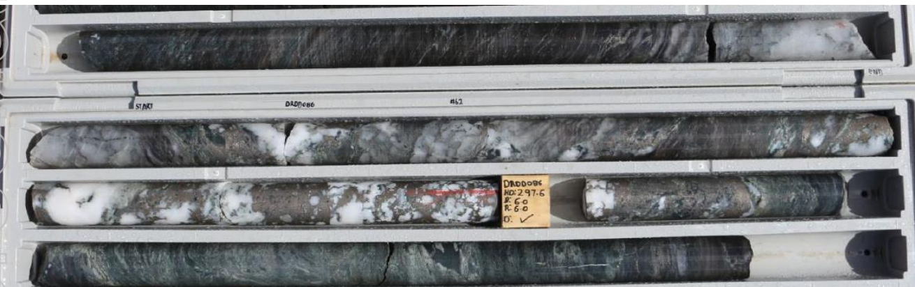
Figure 2: Recent drill hole DRDD086 Bellevue Lode: quartz massive to 20% disseminated pyrrhotite, trace disseminated chalcopyrite lode. Assays pending
