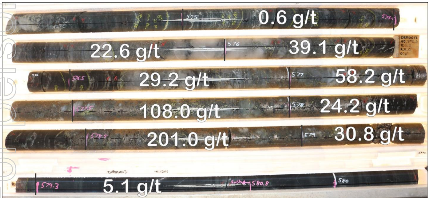
Figure 1: DRDD013 Viago Lode diamond drill core intercept 4.3m @ 58.8 g/t gold at 575.5 m
