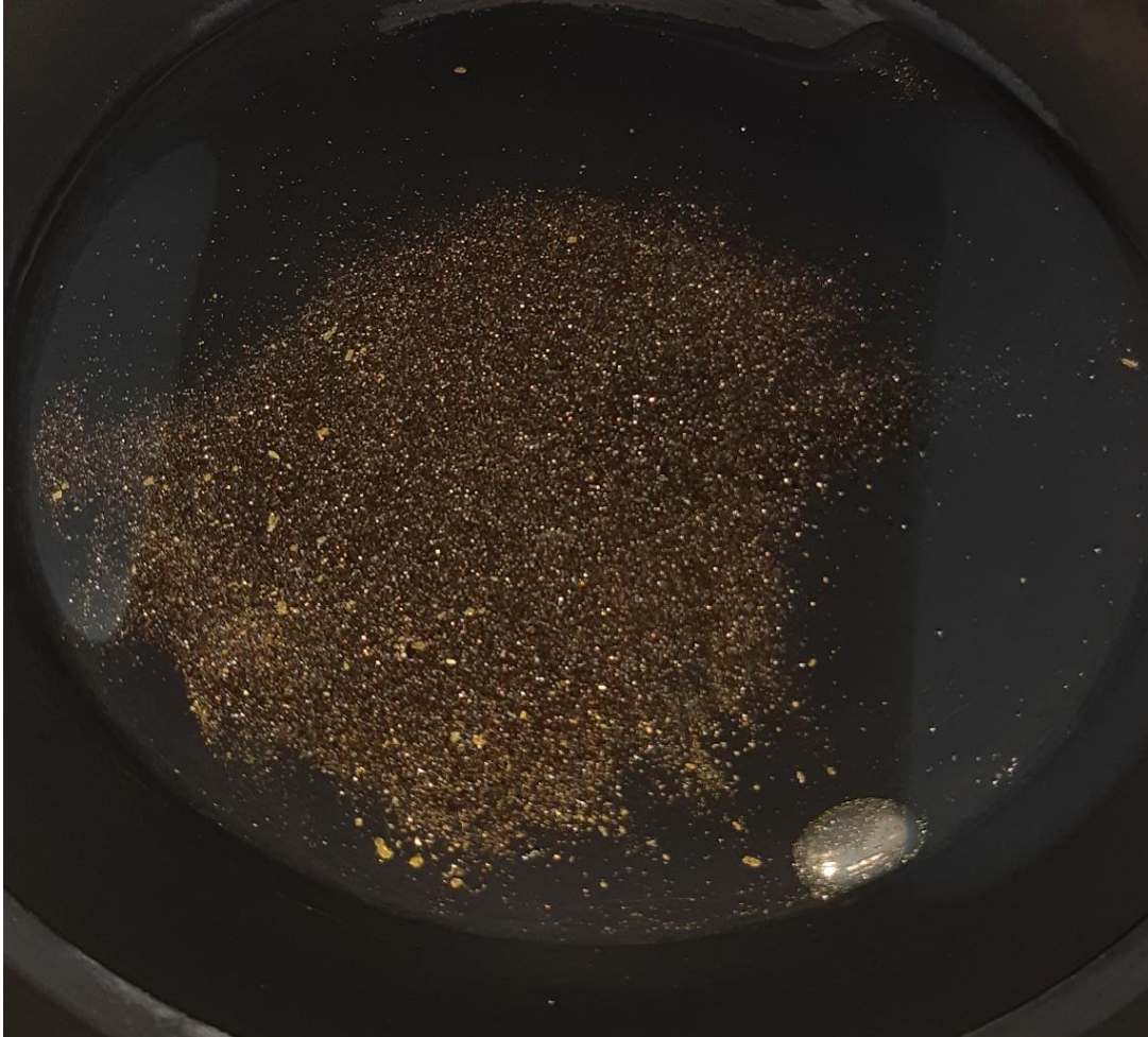
Figure 1: Gravity concentrate recovered from the Viago Lode 10 kg sample showing abundant gold grains
